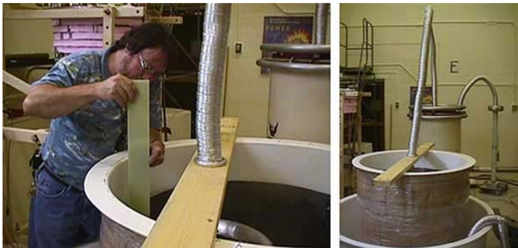
Figure 5. (Left) Alvin Ellis sets the gap between the side wall and a component of the FCL mockup in an open liquid nitrogen bath. The mockup is suspended in the bath which allows changing of the gap and isolation from the bottom of the tank. (Right) Open bath showing the high voltage connections for ac partial discharge testing.
