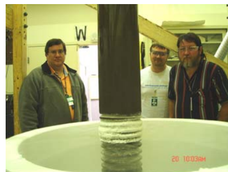
Fig. 3. Left to right, Drew Hazelton and Wayne Ordon of SuperPower and Alvin Ellis of ORNL examine the lower end of the bushing immersed in LN2. Ice formation occurs on the sheds just above the surface of the LN2.
