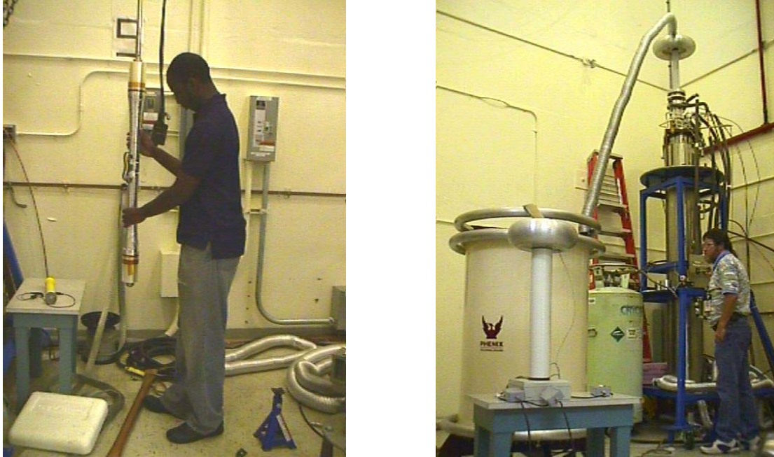
Fig. 15. (left) Technician holding model cable prior to immersion into large high voltage cryostat. (right) AC withstand setup showing the large HV cryostat in the background.
