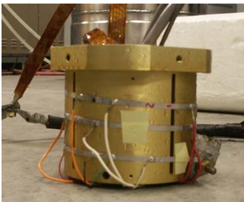
Fig. 24. Experimental setup for splice measurement of YBCO coated conductors and schematic of series of splice joints that was wound on the anodized aluminum mandrel.
