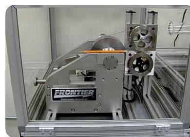
Fig. 1. ORNL reel-to-reel slot die coater for solution deposition.
