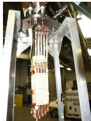
Fig. 1. Front-view of test apparatus used to measure I_c of 2 G YBCO tapes vs. magnetic field and orientation angle ( \theta ).
