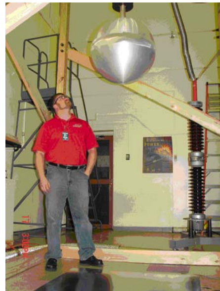
Fig. 2. Wayne Ordon of SuperPower inspects a 22 inch (55.9 cm) diameter aluminum sphere used as a bushing termination for air withstand tests. A large air gap of 60 inches (1.52 m) was required to prevent flashover when qualifying at 650 kV impulse voltages.
